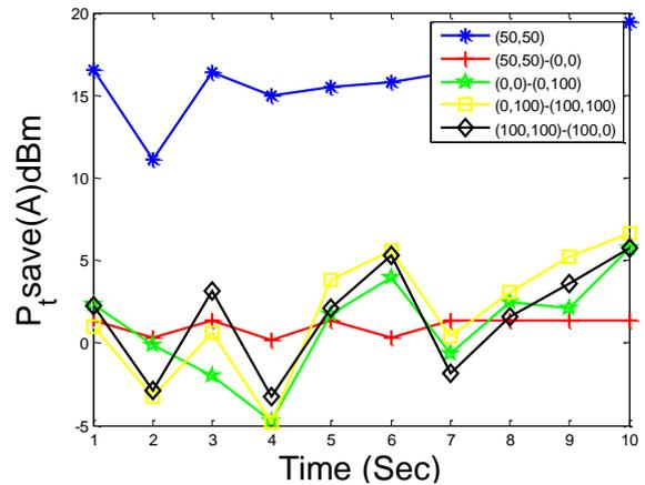
Figure 2: Transmitter power level versus time analysis for region A
