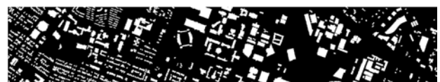
Fig. 5. Classification of the fused LiDAR and hyperspectral data using machine learning method.
