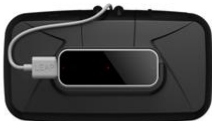
Fig.2 Leap motion controller mounted on Oculus Rift
