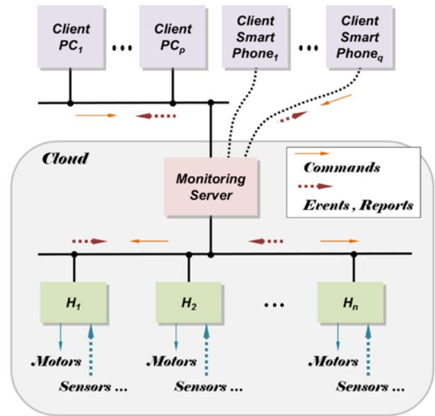
Fig. 1 The framework of multi-agent cloud system of remote housing management.
