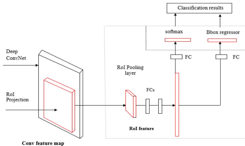
Fig.1 Working model of Fast R-CNN
