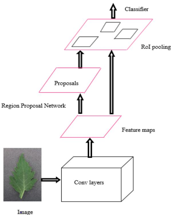
Figure3. Working model of Faster R-CNN with Region Proposal Network
