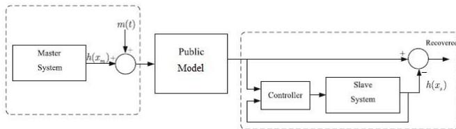
Fig.6. Block Diagram of System Masking Scheme
