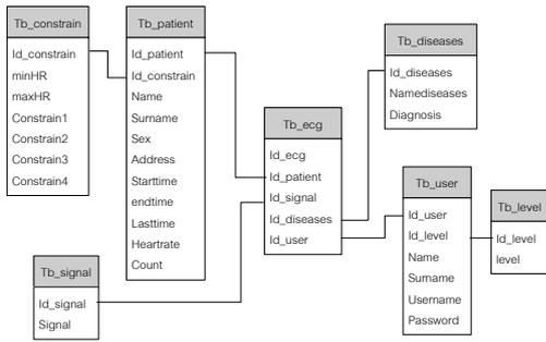
Figure 9. Database of ECG signal processing through WBBNS
