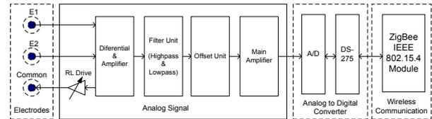
Figure 7. The design of ECG monitoring via WBBN block diagram.
