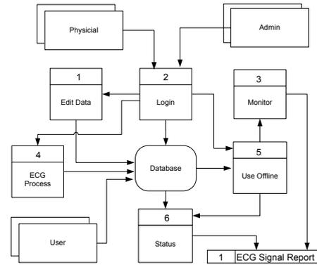
Figure 11. Data Flow Diagram of web services over WBBNS and the internet
