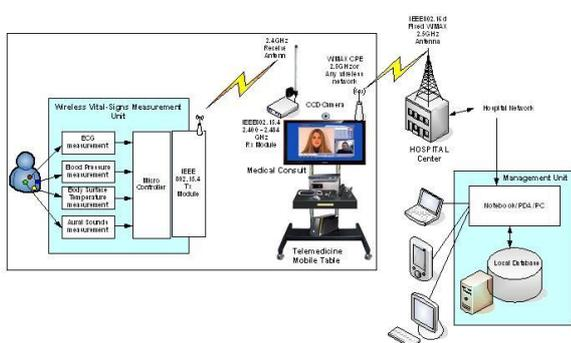
Figure 4. Structure of telemedicine via WBBN
