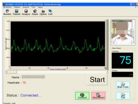
Figure 10. Measurement results are displayed in real time via WiMAX.
