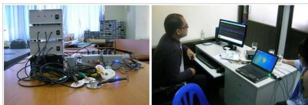
Figure 14. ECG&HS equipment prototype with monitoring via Wi-MAX network.
