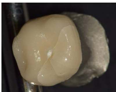
Fig. 6. Fracture initiation point and extension.
