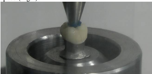
Fig. 2. Probe under loading
