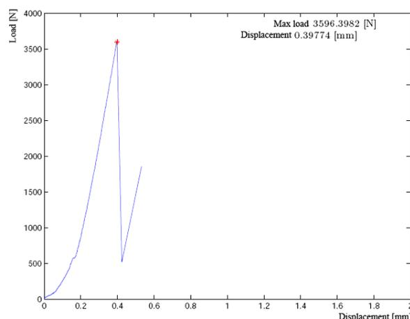
Fig. 3. Graphical representation of the load distribution over time, relative to the displacement for sample 1 (fracture type 4).
