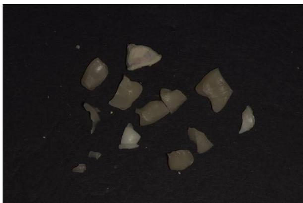
Fig. 6. Fracture pattern of sample 1 – type 4 - with fracture of the framework and veneering material in multiple pieces.
