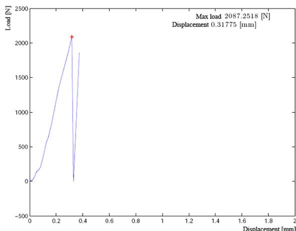
Fig. 5. Graphical representation of the load distribution over time, relative to the displacement for sample 3 (fracture type 3).
