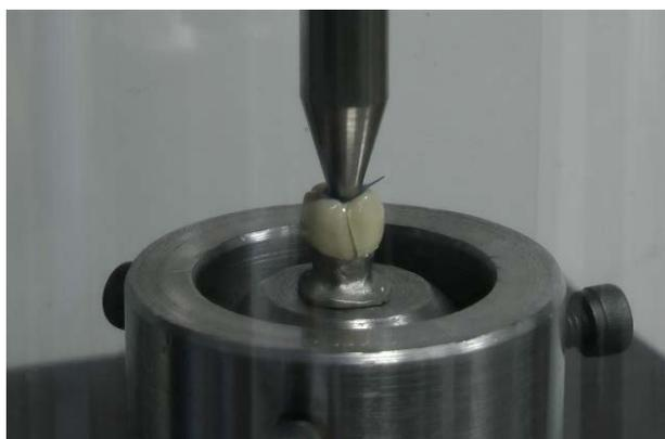
Fig. 1. Compressive loading in the testing device until fracture of the restoration.
