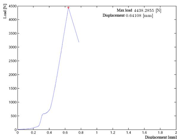
Fig. 7. Graphical representation of the load distribution over time, relative to the displacement for sample 4 (fracture type 4).
