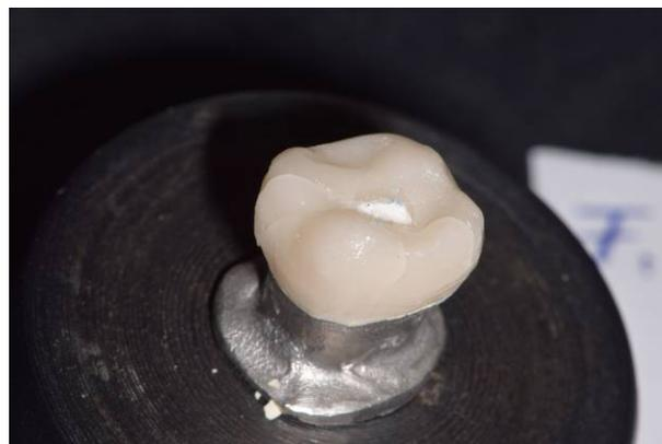
Fig. 2. Fracture pattern of sample 1 – type 4 - with fracture of the framework and veneering material.
