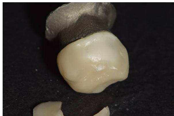
Fig. 4. Fracture pattern of sample 3 – type 3 – fracture of the veneering material, exposing the framework.
