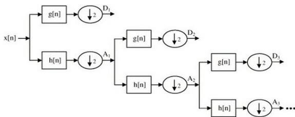
Fig. 2 Discrete wavelet transform process
