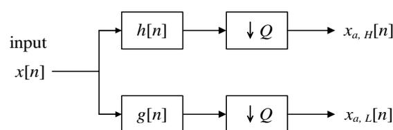
Fig. 1 The structure of Discrete Wavelet Transform
