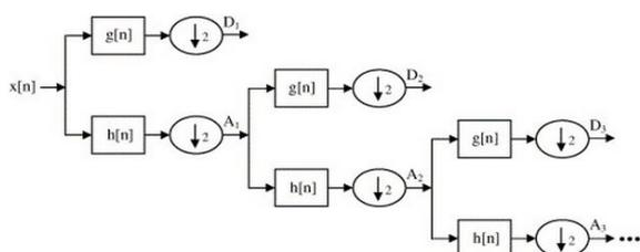
Fig. 2 Discrete wavelet transform process
