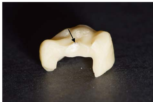
Fig. 1. Fracture surface of a pressed ceramic crown specimen exposing fracture origin on the occlusal loading point and the fractographic map.
