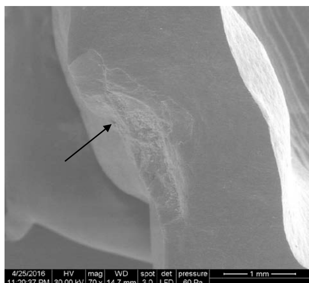
Fig. 1. Fracture surface of a pressed ceramic crown specimen exposing fracture origin on the occlusal loading point and the fractographic map.
