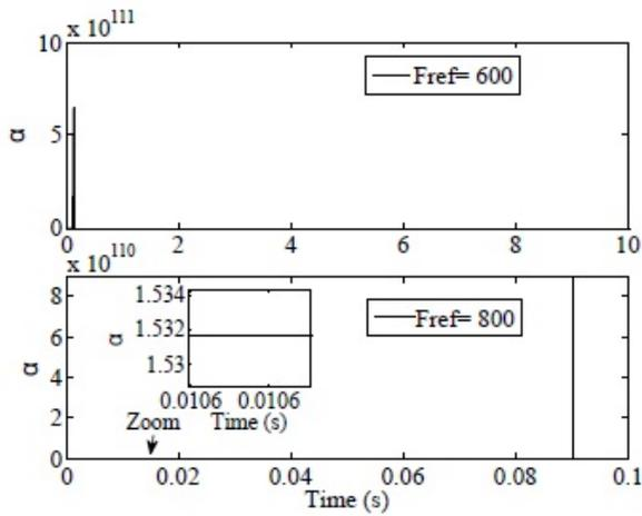
Figure 4: Evolution of the obtained impulse amplitude for the control of the force for  $F_{ref}= 600$  and  $800$  N with  $dt= 10$  ms.
