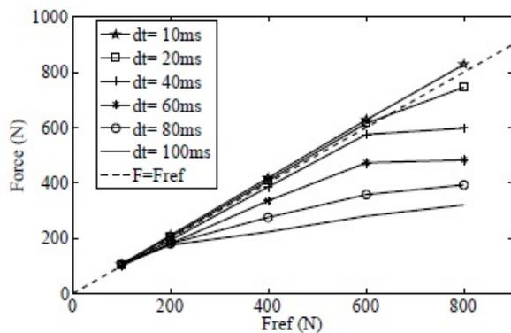
Figure 7: Application of the white noise of 5% for the  $F_{ref}= 100, 200, 400, 600$  and  $800$  N and  $dt= 10, 20, 40, 60, 80, 100$  ms.
