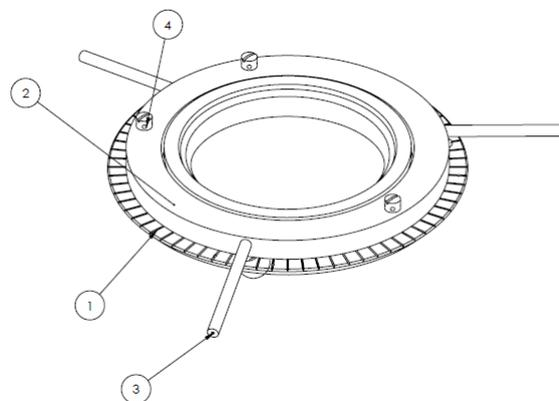
Figure 2: Frame and Drive with Rods and Fiducial Points.
