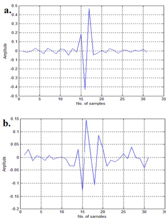
Fig. 3: DWT 3<sup>rd</sup> level detail coefficients a) N beat and b) S beat.
