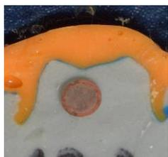
Fig.5. Section through sample prepared for microscope
