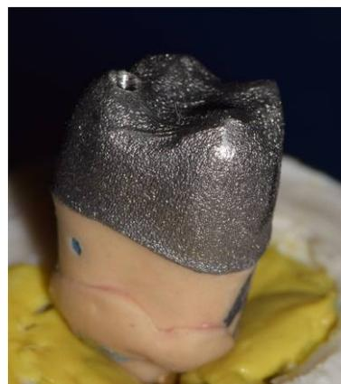
Fig. 5. Framework prepared for fit tests.
