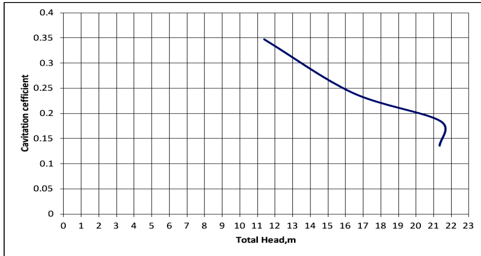
Fig.9 Plot of cavitation coefficient versus total head at 1.6 m suction lift
