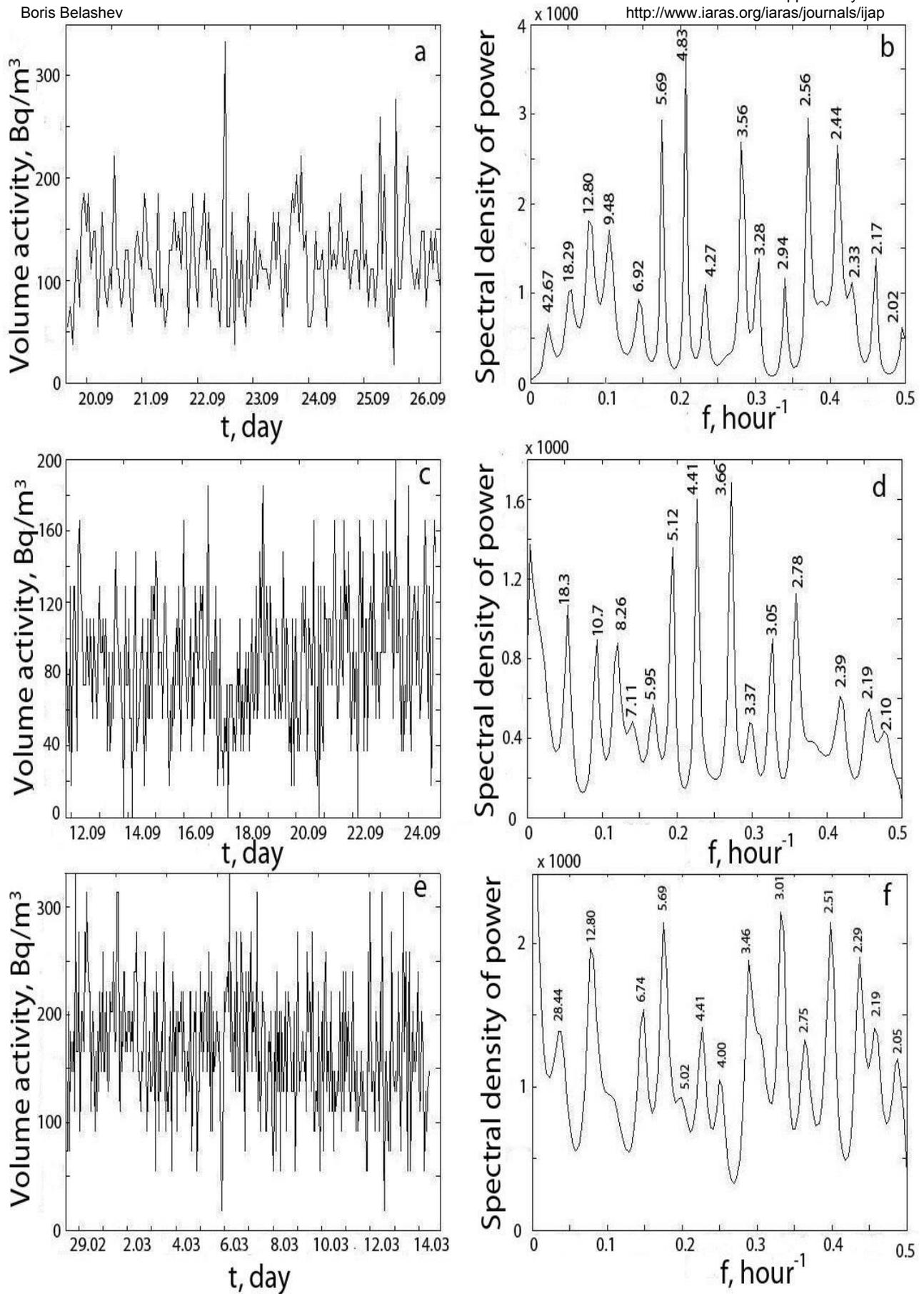
Fig. 3 Volumetric radon activity spectra recorded in the air of basements in the village of Tsarevichi from 20 to 26.09.2016 (a), in Solomennoye Town from 12 to 24.09.2014 (c) and the City of Pitkäranta from 29.02 to 14.03.2016 (e) with a one-hour discretization period and their power spectra (b, d, f), respectively.
