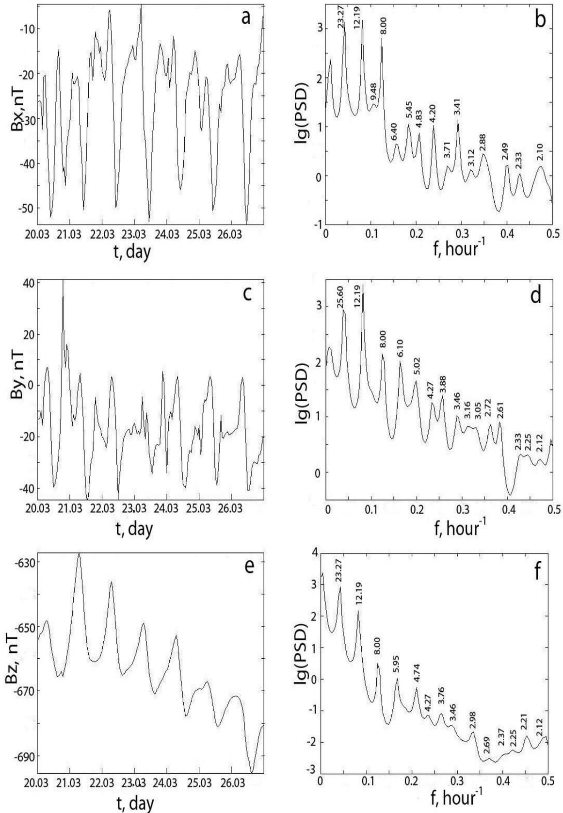
Fig. 2 Variations in three components  $B_x$  (a),  $B_y$  (c),  $B_z$  (e) of a geomagnetic field from 20- to 26.03.2016 with a one-hour discretization period and their power spectra (b, d, f), respectively.
