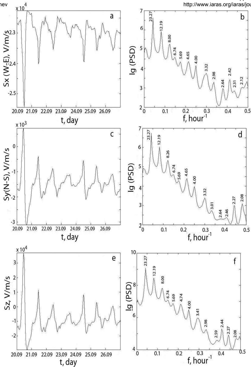
Fig. 1 Seismic noise series of three spatially oriented seismic meters with a one-hour discretization interval (a), (c), (e) and their power spectra (b, d, f), respectively
