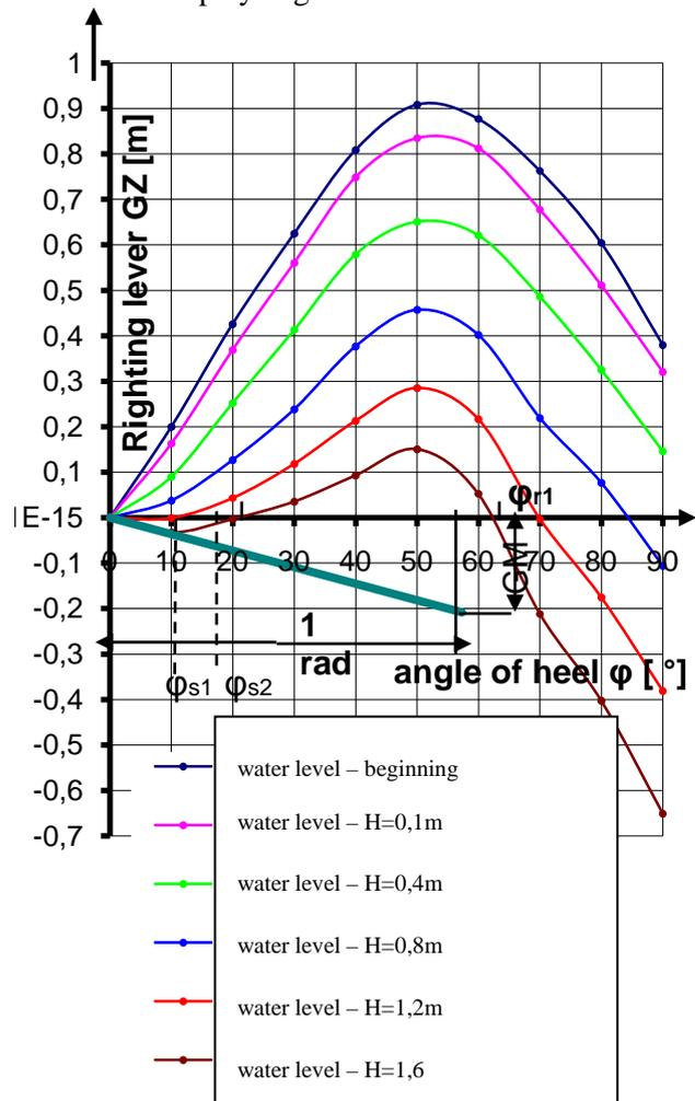
Fig. 4. Influence of the amount of water in the compartment on the Reed's curve
