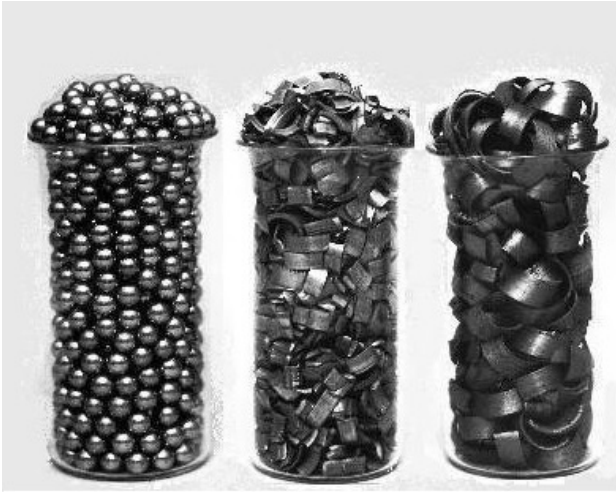
Fig.1 Picture of a filter-matrix in the form of balls and ground chips loadings.
