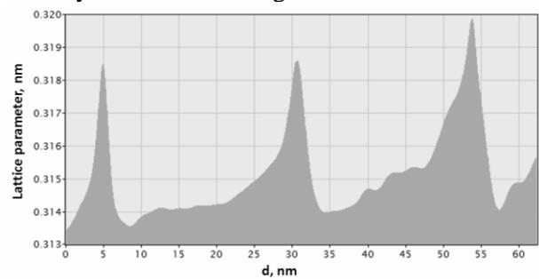
Fig. 4. A profile of the lattice parameter from the film thickness along <111> for the multilayer Ge<sub>0.5</sub>Si<sub>0.45</sub>Sn<sub>0.05</sub>/Si heterostructure.
