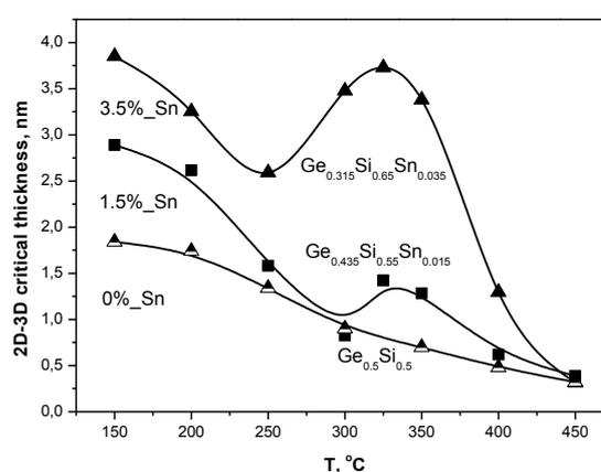
Fig. 1. Temperature dependence of the 2D-3D transition for GeSiSn films with Ge content: 31.5, 43.5 and 50 % for a 2% misfit with Si.
