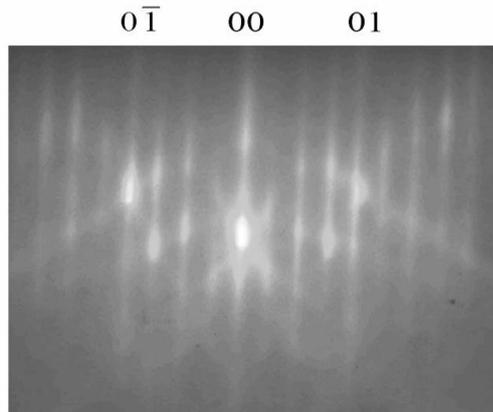
Fig. 2. RHEED pattern along the [110] surface of Si with a superstructure (4 × 4), the coating layer containing GeSiSn c Sn 3.5%
