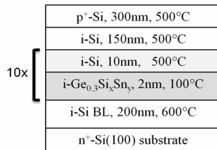
Fig. 5. Scheme of the p-i-n structure.
