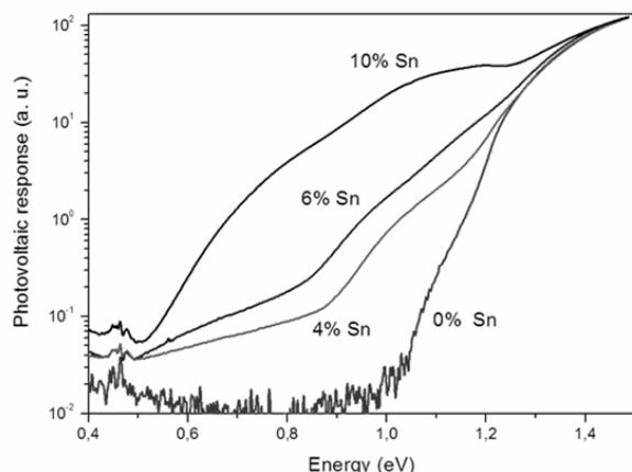
Fig. 6. A series of photoconductivity spectra in the photovoltaic regime at zero bias for the samples with the different Sn content in the p-i-n structure.
