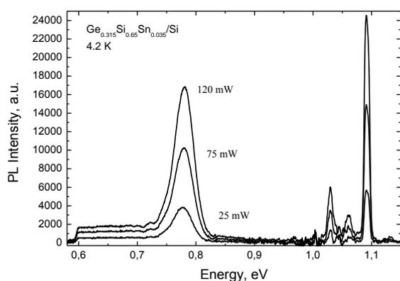
Fig. 7. Photoluminescence spectra obtained at a temperature of 4.2 K for the heterostructure containing 3.5 % Sn.
