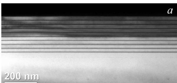
Fig. 3. TEM image of Ge<sub>0.5</sub>Si<sub>0.45</sub>Sn<sub>0.05</sub>/Si heterostructure with period 25 nm.
