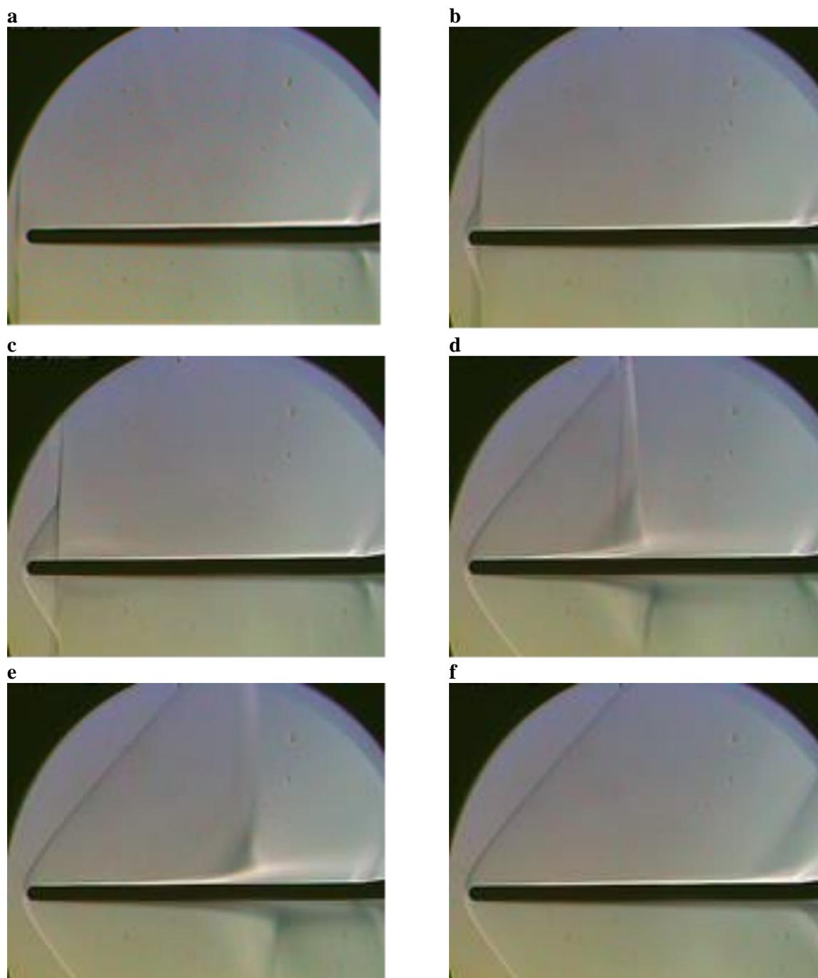
Fig. 3. Photos of shadow visualization illustrated dislocation of normal shock wave along the model in the test section of the wind tunnel with increasing of the total pressure, horizontal model installation.
