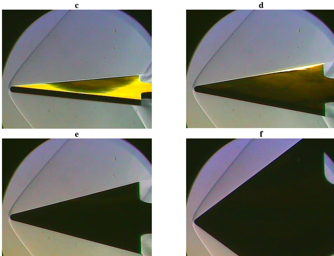
Fig. 5. Examples of shadow visualization of rotated model
