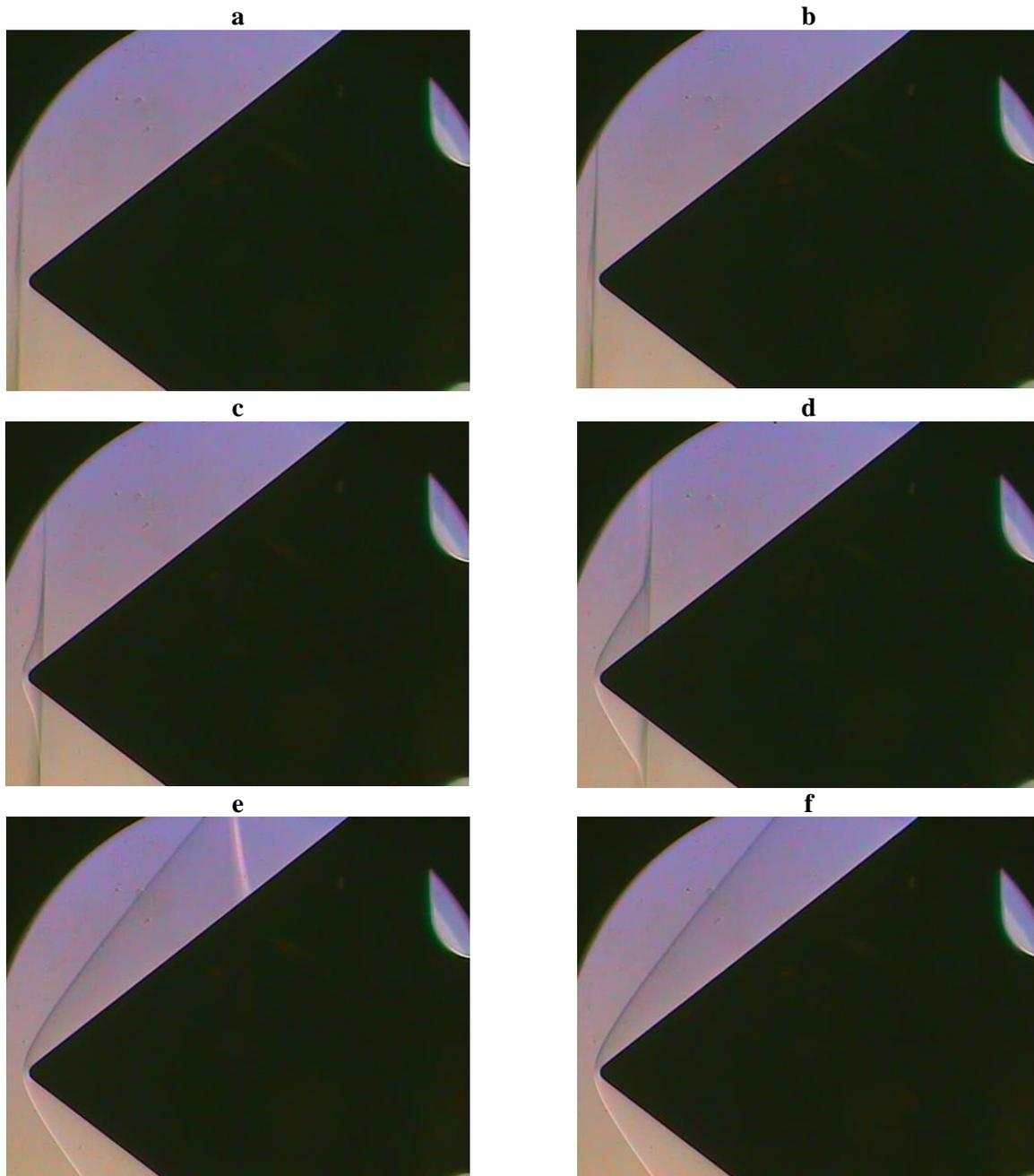
Fig. 4. Photos of shadow visualization illustrated dislocation of normal shock wave along the model in the test section of the wind tunnel with increasing of total pressure, vertical model installation.
