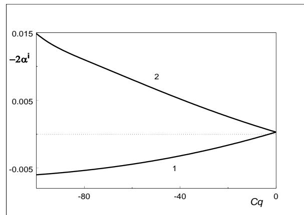
**Fig. 3.** Effect of the injection intensity  $Cq$  on the growth rates of the three-dimensional vortex waves at  $M = 2$ ,  $Re = 600$ ,  $2b = 0.225$ , and  $F = 0.192 \times 10^{-4}$  for the streamwise  $\phi = \pi$  (1) and counterstream  $\phi = 0$  (2) curtains
