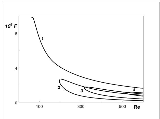
**Fig. 5.** Neutral curves of the vortex mode on thermally insulated surfaces for different  $Cq$  in the case of the normal injection  $\varphi = \pi/2$ ,  $Cq = -0.3$  (curve 1) and the streamwise curtain  $\varphi = \pi$ ,  $Cq = -0.3$ ,  $-50$ , and  $-100$  (2–4).
