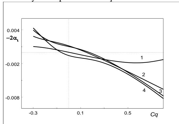
**Fig. 1.** Growth rates of the three-dimensional vortex waves at  $M = 2$ ,  $Re = 600$ , and  $2b = 0.225$  as functions of the mass transfer intensity  $Cq$  for the frequencies  $F = (0.19, 0.38, 0.57, 0.76) \times 10^{-4}$  (curves (1–4)).
