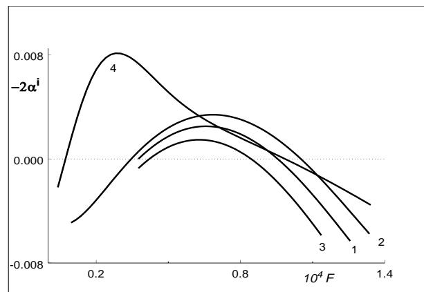
**Fig. 10.** Frequency cuts illustrating the growth rates of three-dimensional disturbances ( $2b = 0.225$ ) at  $Re = 600$  and  $Cq = -50$ ; for the streamwise curtain the same parameters as in Fig. 9 and for the counter-stream curtain thermally insulated wall with  $T_w = 1.889$  (4).
