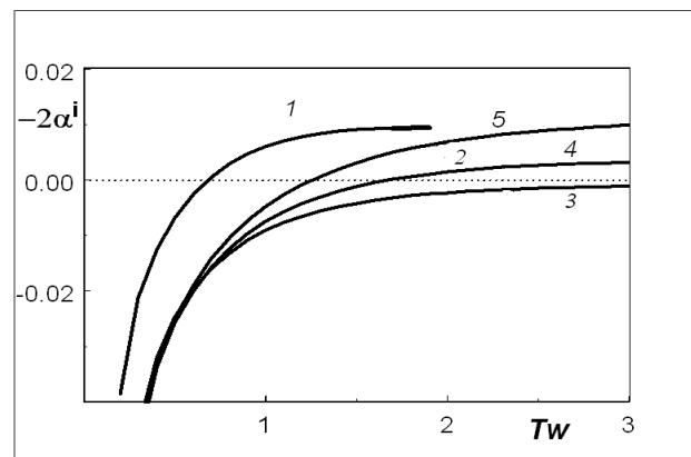
**Fig. 8.** Temperature ( $T_w$ ) dependence of the three-dimensional disturbance growth rates ( $2b = 0.225$ ) at  $Re = 600$  and  $F = 0.192 \times 10^{-4}$  in the case of the normal injection ( $Cq = -0.3$  and  $\varphi = \pi/2$ , curve 1) and at  $Cq = 0.3$  and  $-50$  for the streamwise (2, 3) and counterstream (4, 5) curtains.
