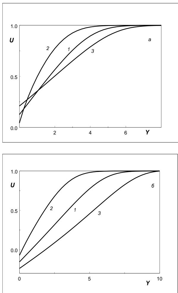
**Fig. 7.** Effect of the temperature factor on the mean velocity profiles at  $Cq = -50$  for different streamwise (a) and counterstream curtains (b); (1) thermally insulated wall, (2) cooling, and (3) heating.
