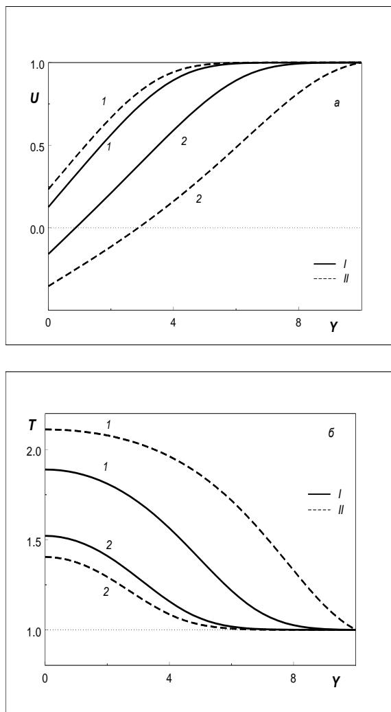
**Fig. 4.** Effect of the curtain angle and the injection intensity  $Cq$  on the profiles of the mean longitudinal velocity (a) and the mean temperature (b) for  $Cq = -50$  (I) and  $-100$  (II); (1, 2) correspond to  $\varphi = \pi$  and 0.
