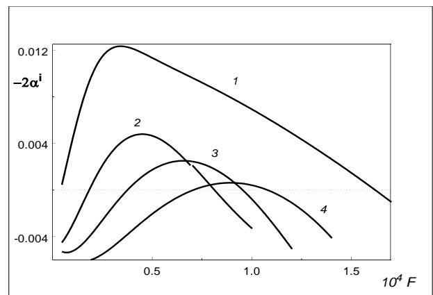
**Fig. 6.** Frequency cuts illustrating the growth rates of three-dimensional disturbances ( $2b = 0.225$ ) at  $Re = 600$  and the same parameters as in Fig. 5
