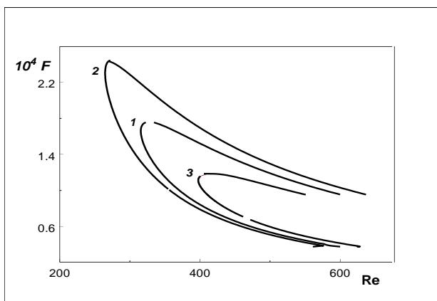
**Fig. 9.** Neutral curves of the vortex mode on noninsulated surfaces for the streamwise curtains at  $Cq = -50$  in the case of heating ( $T_w = 1.62$ , 2) and cooling ( $T_w = 1.42$ , 3) in comparison with the case of the thermally insulated wall ( $T_w = 1.52$ , 1).
