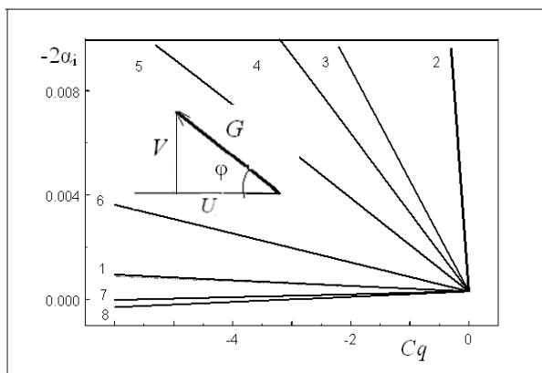
**Fig. 2.** Effect of the angle  $\phi$  of inclination of the injected gas velocity on the growth rates of the three-dimensional vortex waves at  $M = 2$ ,  $Re = 600$ ,  $2b = 0.225$ , and  $F = 0.192 \times 10^{-4}$ ; (1–8) relate to  $\phi = 0, 1.57, 3.0, 3.04, 3.08, 3.12, 3.14$ , and  $3.1416$ ; in the same figure the schematics of the arrangement of the longitudinal  $U$  and normal  $V$  velocity components are presented.
