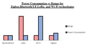
Figure 4: Power Consumption vs. Range for Bluetooth/LE, LoRaWan, and Wi-Fi technologies
