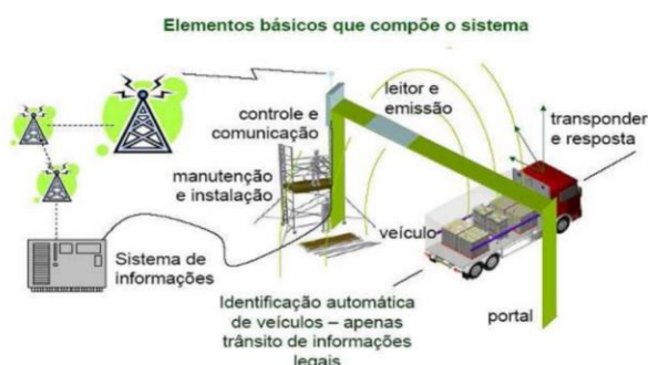
Fig. 1: Basic elements that make up the system
