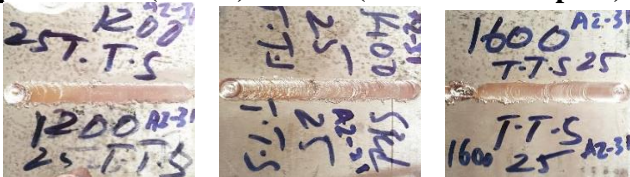
Fig.4.a.the weld made at 1200RPM at 25 Tool traverse Speed with similar welding Az31alloy ,Fig.4.b. the weld was made at 1400RPM at 25 Tool traverse Speed with similar welding Az31alloy ,Fig.4.c. the weld made at 1600RPM at 25 Tool traverse Speed with similar welding Az31alloy
