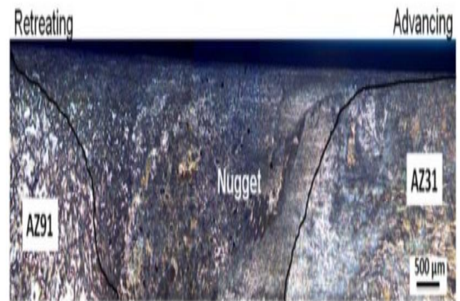
Fig.9.Microstructure taken at cross section of Welding process at low magnification dissimilar welding processAz-91/Az-31
