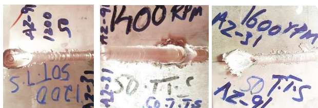
Fig.(12.a)the weld made at 1200RPM at 50 Tool traverse Speed with Dissimilar welding Az91/Az31alloy, Fig.12.b. the weld was made at
