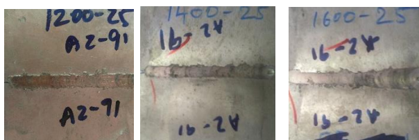
Fig.6.a.the weld made at 1200RPM at 25 Tool traverse Speed with similar welding Az91alloy, Fig.6.b. the weld was made at 1400RPM at 25 Tool traverse speed with similar welding Az91ally, Fig.6.c. the weld was made at 1600RPM at 25 Tool traverse Speed with similar welding Az91alloy
