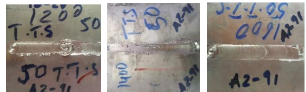
Fig.7.a.the weld made at 1200RPM at 50 Tool traverse Speed with similar welding Az91alloy, Fig.7.b. the weld was made at 1400RPM at 50 Tool traverse speed within stir welding Az91ally, Fig.7.c. the weld was made at 1600RPM at 50 Tool traverse Speed with similar welding Az91alloy
