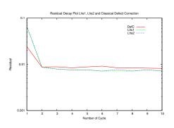
Figure 7: Comparison of residual decay of EHL by splitting  $L_{hs1}$ , splitting  $L_{hs2}$  and classical Defectcorrection at  $\kappa = 0.0$  on 7<sup>th</sup> level V(2, 1) cycle
