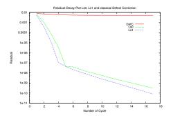
Figure 5: Comparison of residual decay of splitting *Ls*0 and splitting *Ls*1 for  $\kappa = 1/3$  on 7<sup>th</sup> level *V*(2,1) cycle
