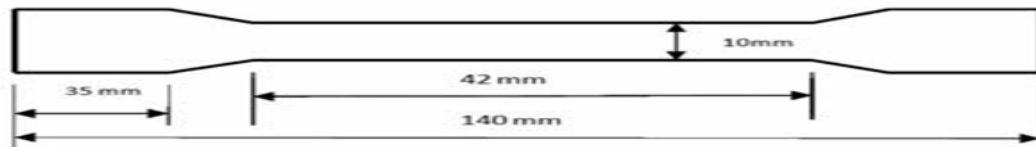
Figure:-2 A specimen for tensile test
