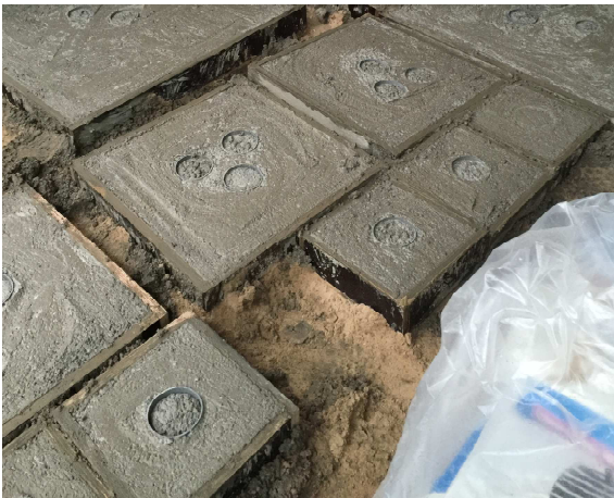
Fig.5. Specimen sets cured in 300x300mm moulds
