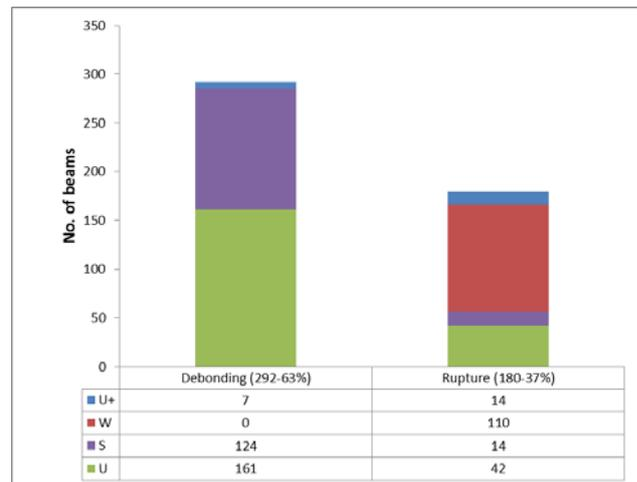
Fig.3 Modes of failure in beams using different FRP configurations
