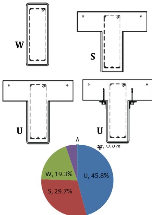
Fig.2. Shear Strengthening of EBFPR Beams:
