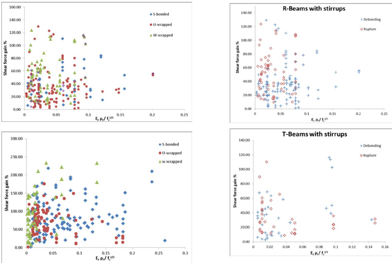
Fig.4 Shear force gain versus  $E_f \rho_f / f_c^{2/3}$  ratio for different FRP configurations a) With stirrups, b) Without Stirrups
