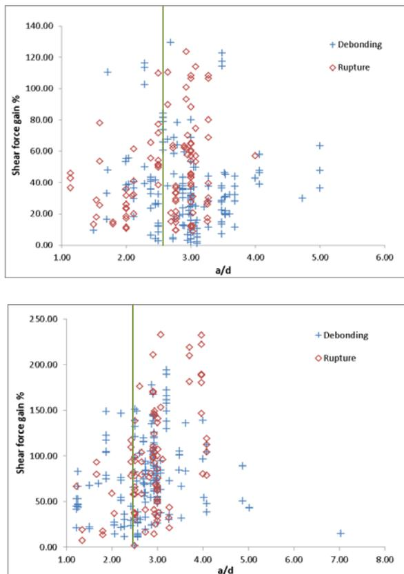
Fig.6 Shear force gain versus the shear span to depth ratio ( $a/d$ ) for (a) beams with stirrups and (b) without stirrups
