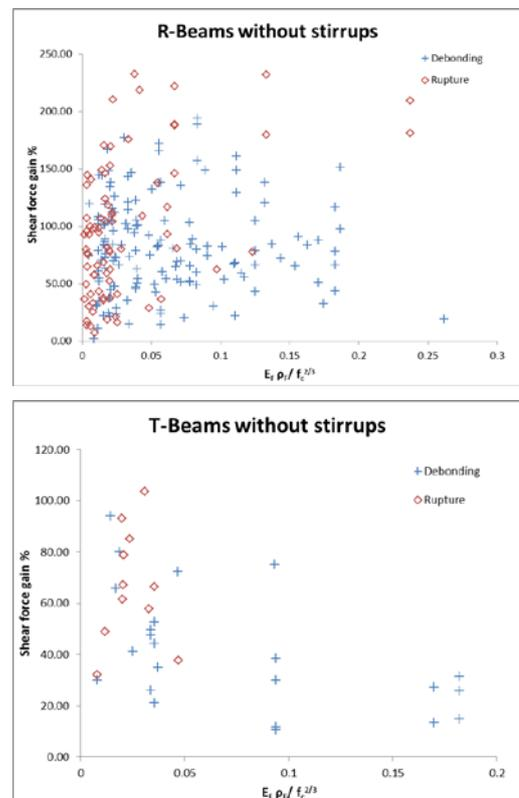
Fig.5 Shear force gain versus  $E_f \rho_f / f_c^{2/3}$  in beams with and without stirrups for different cross section types
