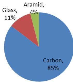
Fig.1. Distribution of Type of Fibers used in EB FRP Beams
