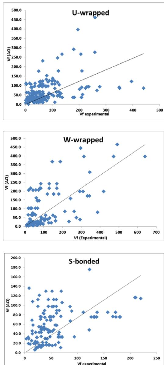
Fig.7 Predictions of the ACI design model for S-bonded, U-wrapped and W-wrapped EBFPR RC beams.
