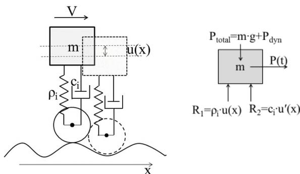
Fig. 1 A spring-mass-damper-system in railway engineering: (left) a railway vehicle on a railway track with longitudinal defects and (right) the forces exerted on the "car-body".
