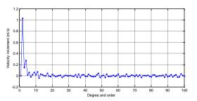
Figure 1- Difference between the velocity variation applied to the spacecraft with N +1 and considering only N terms of lunar potential.
