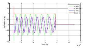
Figure 23 - Thrust applied to the satellite during the simulation without orbital correction.
