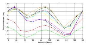
Figure 3 - Velocity variation provided by the disturbance as a function of the inclination of the orbit of the satellite and the number of terms considered for the lunar potential for the first 10 terms.
