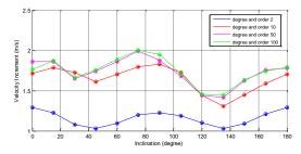
Figure 2 - Velocity variation provided by the disturbance as a function of the inclination of the orbit of the satellite and the number of terms considered for the lunar potential.
