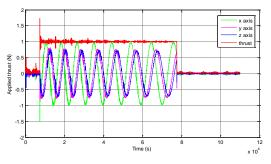
Figure 24 - Thrust applied to the satellite during the simulation with orbital correction.
