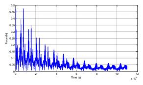
Figure 22 - Perturbations due to the lunar gravitational potential during simulations 3 and 4.
