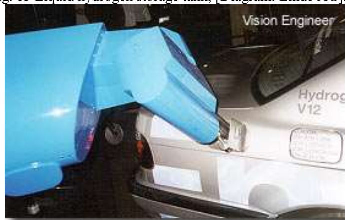
Fig. 16 A Robotic Arm Refilling Liquid Hydrogen to a BMW 5 Series Hydrogen Car, [Simulation], [42]
