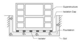
Fig.9: Components of a Base Seismic Isolated Structure, [16].
