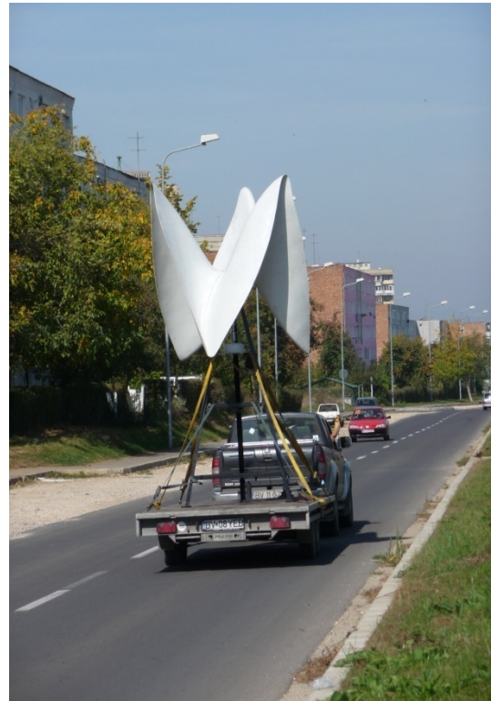
Fig.1 Wind turbine with vertical axis helical type mounted on a car during experimental tests.
