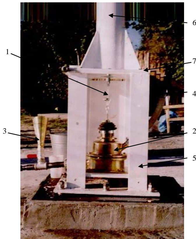
Fig.2 Diaphragm pump used to pump water.
