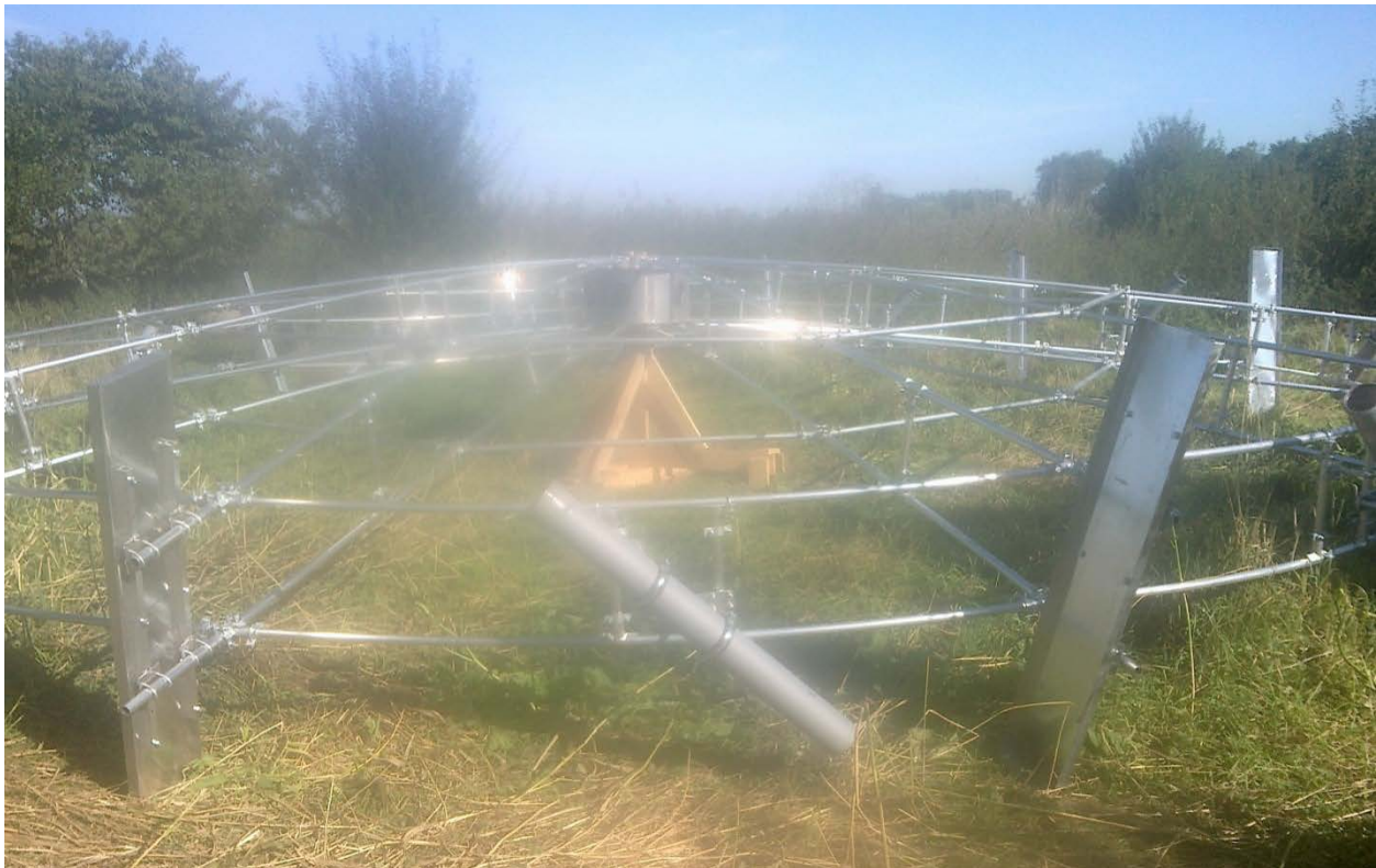
Fig.5 Rotor of a water wheel with a diameter of 10 m.
