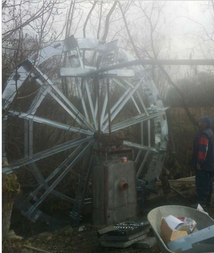
Fig.3 Undershot water wheel used for irrigation of dry lands.
