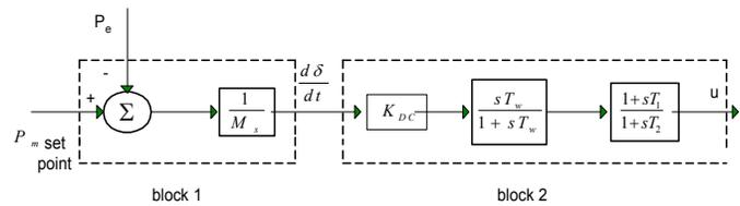
Fig. 3: Structure of Power Oscillation Damping [POD] controller
