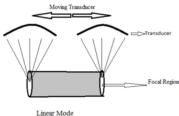
Fig 2: Linear mode of ablation.
