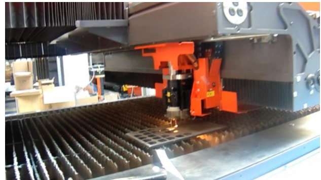
Fig.1 Carbon dioxide laser cutting Hardox 400 samples
