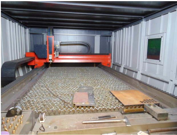
Fig. 2 Fiber Laser and Hardox400 steel plate
