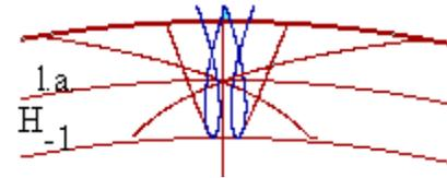
Fig. 7 Path of contact in the section plane  $H_{-1}$
