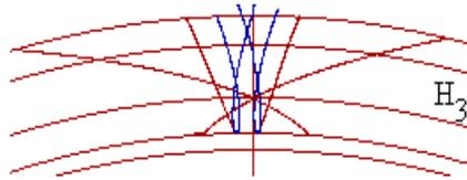
Fig. 4 Path of contact in the section plane  $H_3$
