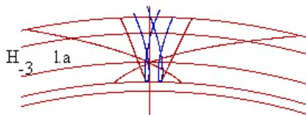
Fig. 3 Path of contact in the section plane  $H_{-3}$
