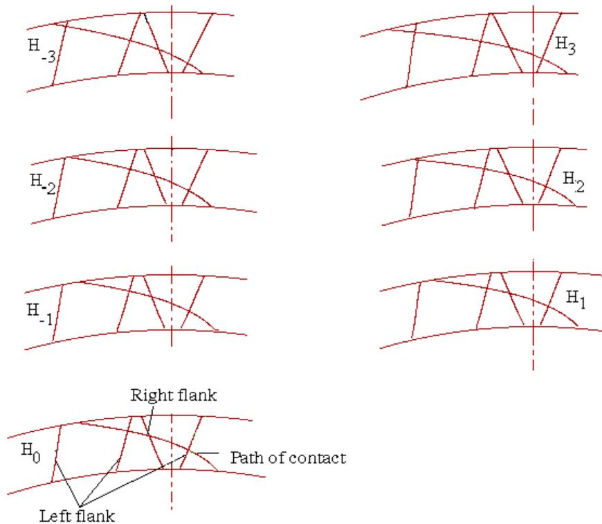
Fig. 9 Contact ratio in the section planes of the worm gear
