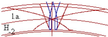
Fig. 5 Path of contact in the section plane  $H_2$
