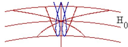
Fig. 2 Path of contact in the section plane  $H_0$
