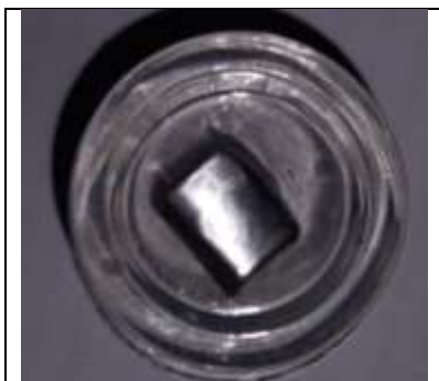
Figure 10.B AISI 1040 After Heat Treatment
