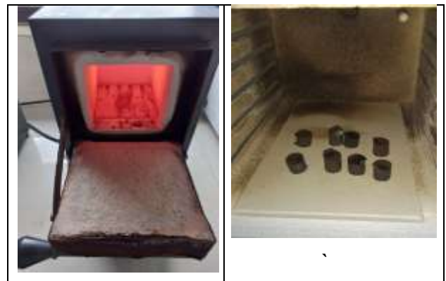
Figure 8. Heat Treatment process AISI 1040 steel specimens at 900°C.
