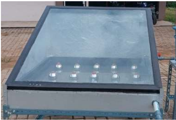
Fig 4. Pictures of each experiment for a solar still desalination device equipped with Phase change material (PCM)
