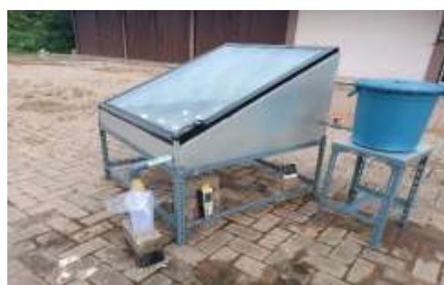
Fig. 1. Solar desalination device with PCM
