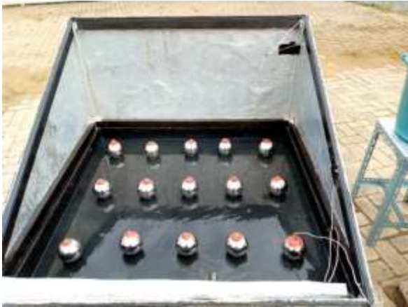
Fig . 4. The ball filled with PCM is placed in the basin
