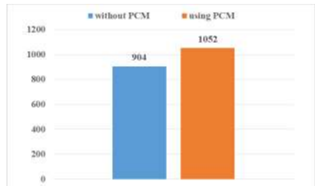
Fig.15 Comparison of the average amount of fresh water produced from 3 experiments without PCM and 3 experiments using PCM
