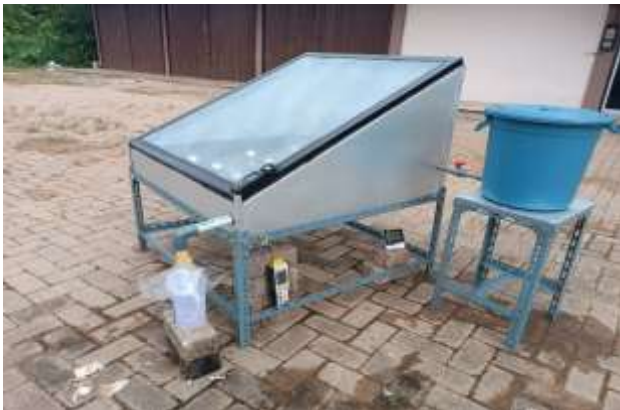
Fig.6 Seawater desalination equipment
