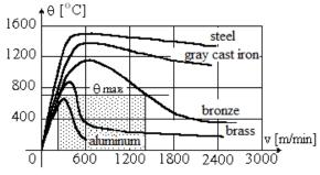
Figure 10 Influence of cutting speed on cutting temperature
