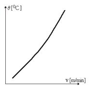
Figure 13 Temperature variation with cutting speed
