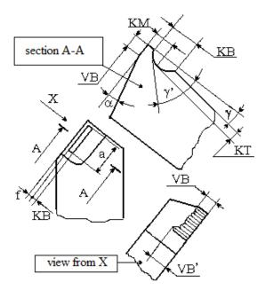
Figura 2 The wear of the edge of a cutting tool
