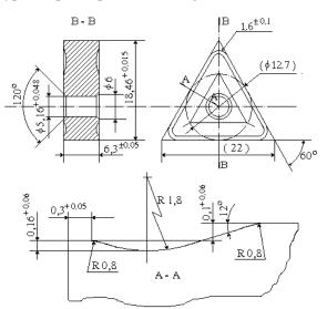
Figure 11 Replaceable plate TNMG, Material groups P and K
