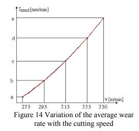
With the data obtained by physical-mathematical modeling of the thermal state in the cutting area, the temperature dependence as a function of velocity can be expressed mathematically through a relation of form:
