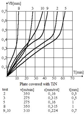
Figure 12 Wear VB of the plates when turning the steel
