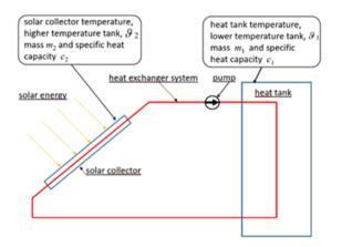
Fig. 1. Scheme of thermodynamic process of heat transfer from the collector to the heat tank
