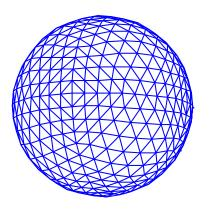
Fig.4 Example of a polyedral patch surface obtained from an 11-frequency tesselated octahedral triangle using the tripetal subdivision of the spherical triangle.
