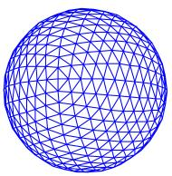
Fig.5 Patched polyedral surface obtained from an 11-frequency tesselated octahedral triangle using the concentric subdivision of the spherical triangle.
