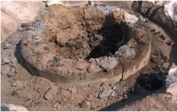
Fig. 2 Reactor lining with melted fuel parts and visible crack
