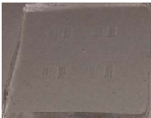
Fig. 7: PDMS printing plate
