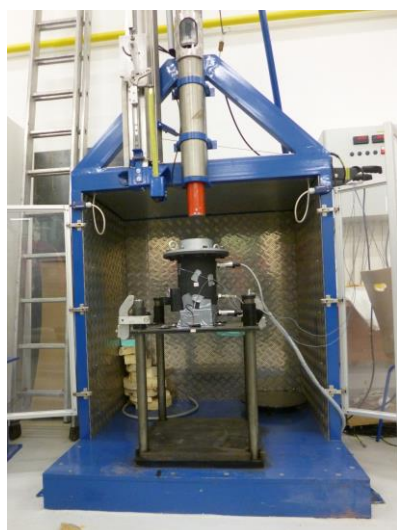
Pic. 3: Accelerating device used for eCall unit testing
